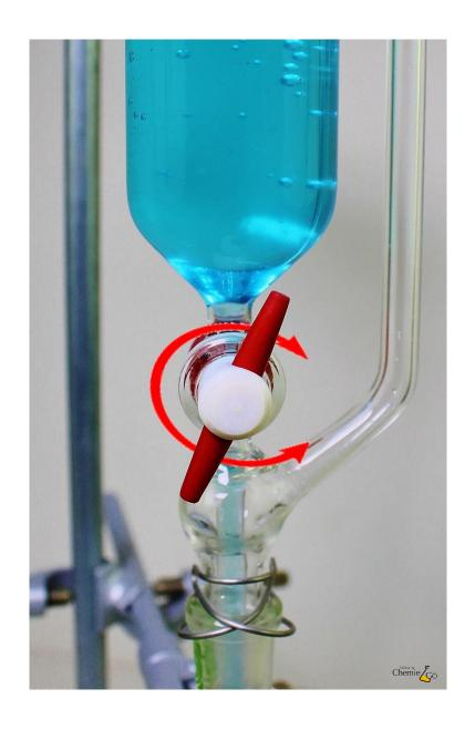
The addition can be adjusted via the valve.
