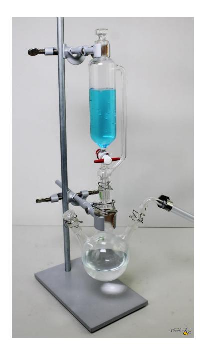
After attaching the joint clamp, the valve is closed and the dropping funnel filled.
