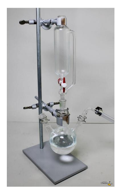
The dropping funnel is secured with a support clamp at the top ground glass joint and connected to the apparatus.
